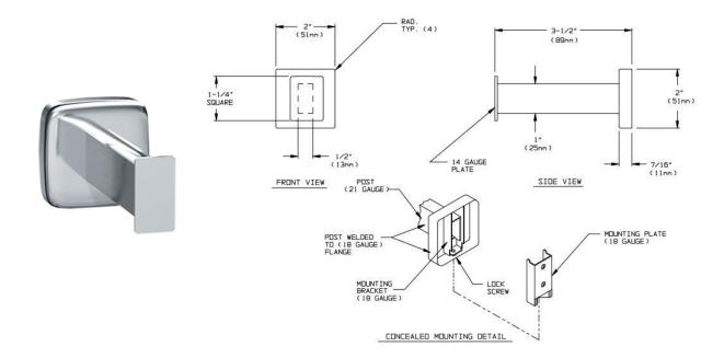
Model WA7301-S is a wall mounted stainless steel towel . Manufactured from grade 304 stainless steel with a satin finish. Supplied complete with rectangular tubing with formed mounting flange and bracket.
